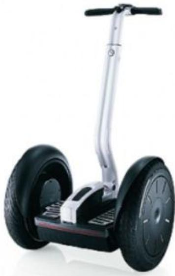
$$\begin{bmatrix} \ddot{x} \\ \ddot{\Phi} \end{bmatrix} = \begin{bmatrix} 0 & \frac{1}{I(M+m) + Mml^2} & 0 & 0 \\ 0 & \frac{-(I+ml^2)b}{I(M+m) + Mml^2} & \frac{m^2gl^2}{I(M+m) + Mml^2} & 0 \\ 0 & 0 & 0 & 1 \\ 0 & \frac{-mlb}{I(M+m) + Mml^2} & \frac{mgl(M+m)}{I(M+m) + Mml^2} & 0 \end{bmatrix} \begin{bmatrix} x \\ \dot{x} \\ \Phi \\ \dot{\Phi} \end{bmatrix} + \begin{bmatrix} 0 \\ \frac{I+ml^2}{I(M+m) + Mml^2} \\ 0 \\ \frac{ml}{I(M+m) + Mml^2} \end{bmatrix} u$$
